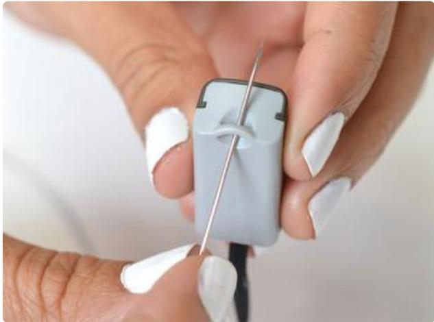
Start with the battery pack. Thread a needle with clear thread (black shown in this step for visibility), double it over on itself, and tie the ends together in a knot.
