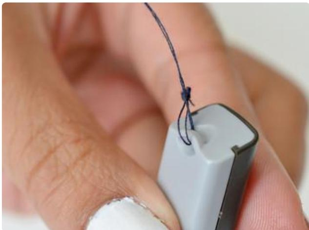
Separate the doubled thread and pull the needle between them, then pull the thread taut. Now the thread is looped securely around the battery pack!
