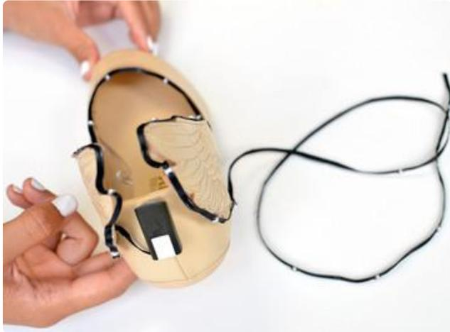
Prototype your design with double-stick tape. This way you can decide where your battery pack will go, and the path your ribbon will take along the shoe, and you can easily readjust as necessary.
