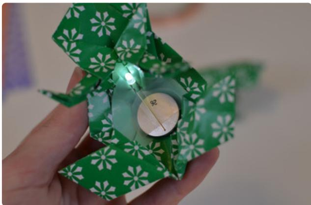
If you're making a pond scene with ITO as described on the next page (<https://adafruit.it/c6n>), prepare the led by taping it inside the frog with copper tape that extends from each lead to the rear feet.
