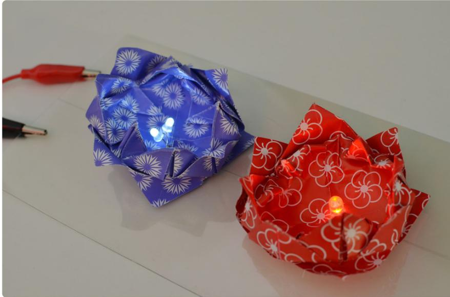
To create a pond for your flowers and frogs, score a piece of [indium tin oxide-coated plastic \(ITO\)](http://adafru.it/1309) down the middle with the blade of a pair of scissors, a craft knife turned sideways, or another sharp-but-not-too-sharp tool to create two conductive planes. Use alligator clips to attach one plane to power and one plane to ground of a battery pack.
