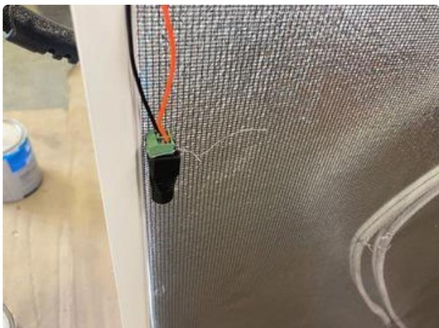
Use screw terminals at the end of your wires - red to + and black to -. I got mine wired so I only needed one screw terminal, but if you get a handful of them and [some power cord splitters \(\)](#), you can use one for each neon strip to make this a no-solder project.
