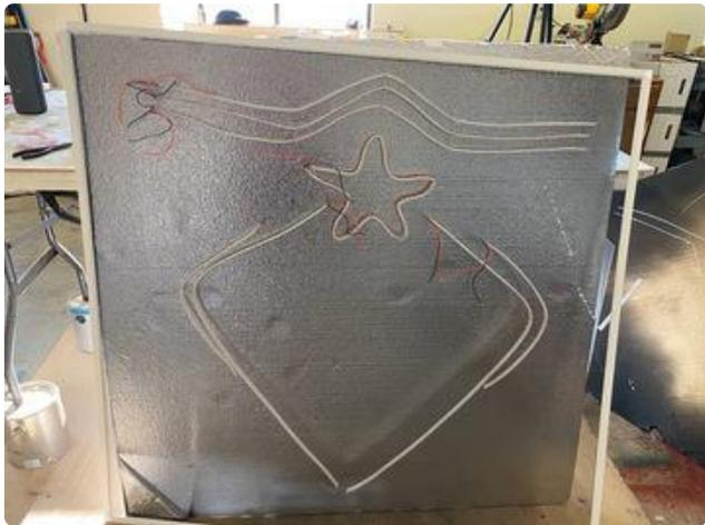
Poke all the neon wires through to the back of your sign. If you've got a soldering iron, put it to use splicing extra lengths of wire between the neon strips. Your wires will show through so be as tidy as you can. It's very possible to hide all the wires behind the neon strips with a little extra wire and effort, if you want it to be perfect.
