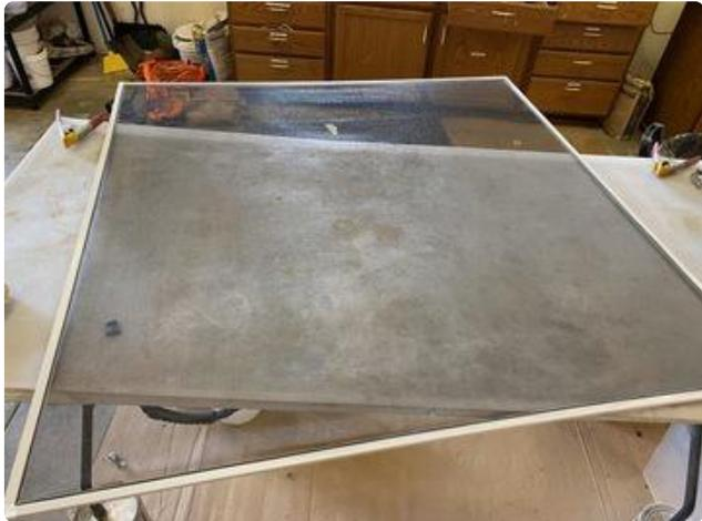
Take your time and try to get nice even tension on the screen the whole way around. Trim off any excess screen sticking out of the groove.
