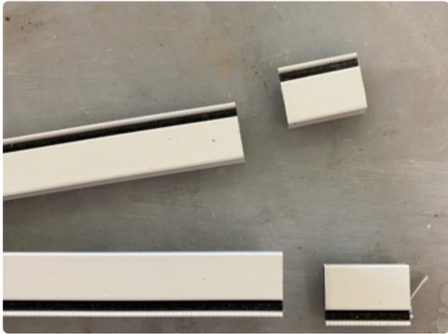
Even though my frame was 48x48, and my screen material roll was 48" wide, I still needed to trim 1" off my frame, because installation requires a bit of overlap with the frame and the 48" screen fabric didn't quite reach. Use a hack saw or a chop saw or whatever you have to get a clean cut.
