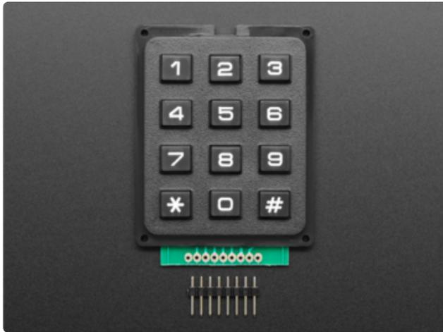
This example is for a 3x4 matrix, such as the Adafruit [3x4 Matrix Keypad \(\)](#) (pictured), the [Adafruit Membrane 3x4 Keypad \(\)](#), or the [3x4 Phone-style Matrix Keypad \(\)](#). For details about wiring these keypads, see the [Matrix Keypad Guide \(\)](#).
