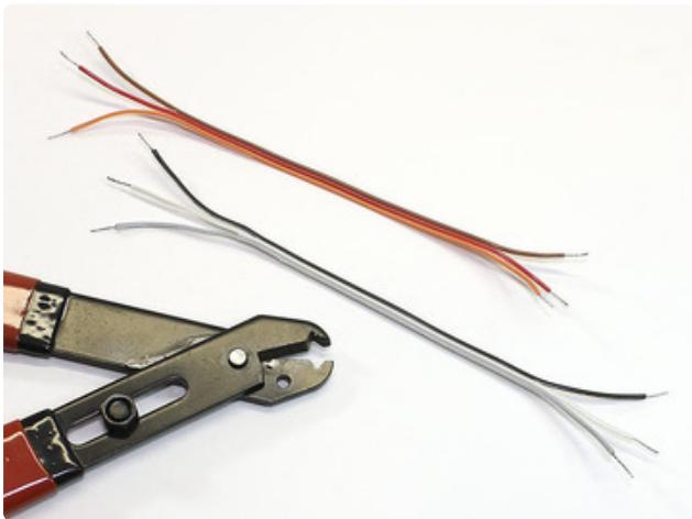
Separate the wires by about **1 inch at both ends**, strip away a little insulation and give the wires a twist to prevent fraying. Optionally tinning the wire ends makes them a little more manageable...heat each one with a soldering iron and melt just a tiny bit of solder into the strands.
