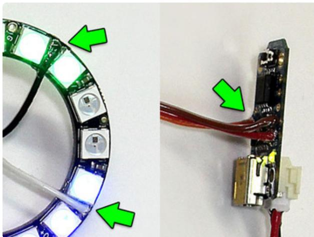
Wait until the glue or epoxy is fully cured before final assembly or charging the battery.
