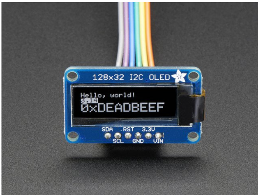
Monochrome 128x32 I2C OLED graphic display
