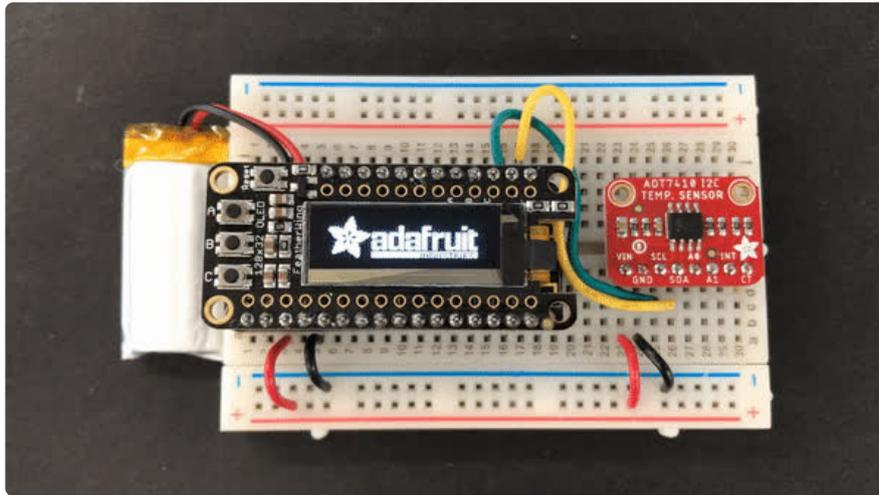
Analog Devices, known for their reliable and well-documented sensor chips - has a high precision and high resolution temperature sensor on the market, and we've got a breakout to make it easy to use! The **Analog Devices ADT7410** gets straight to the point - it's an I2C temperature sensor, with 16-bit 0.0078°C temperature resolution and 0.5°C temperature tolerance. Wire it up to your microcontroller or single-board computer to get reliable temperature readings with ease
