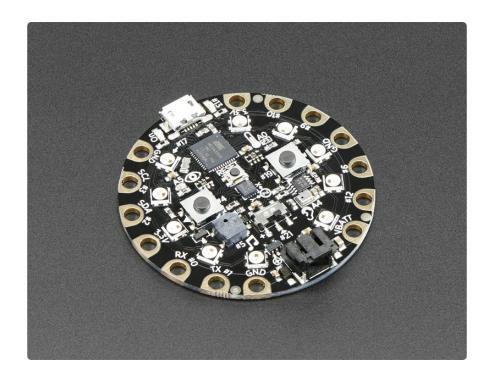
Circuit Playground has built-in USB support. Built in USB means you plug it in to program it, it just shows up - all you need is a Micro-B USB cable, no additional purchases are needed! With the new 1.6.4+ Arduino IDE, it takes only a few seconds to add support (https://adafru.it/nb4). The Circuit Playground has USB HID support, so it can act like a mouse or keyboard to attach directly to computers.
