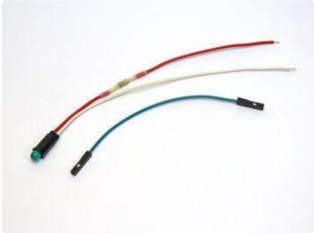
Add wire leads long enough to reach across the camera. Insulate any connections with heat-shrink tube.
