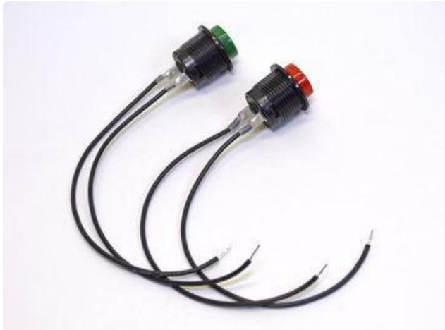
If using the Perma-Proto approach, do not solder everything together yet! Wires can be soldered at the button end, but leave the other end unconnected until all the parts are fitted into the case.
