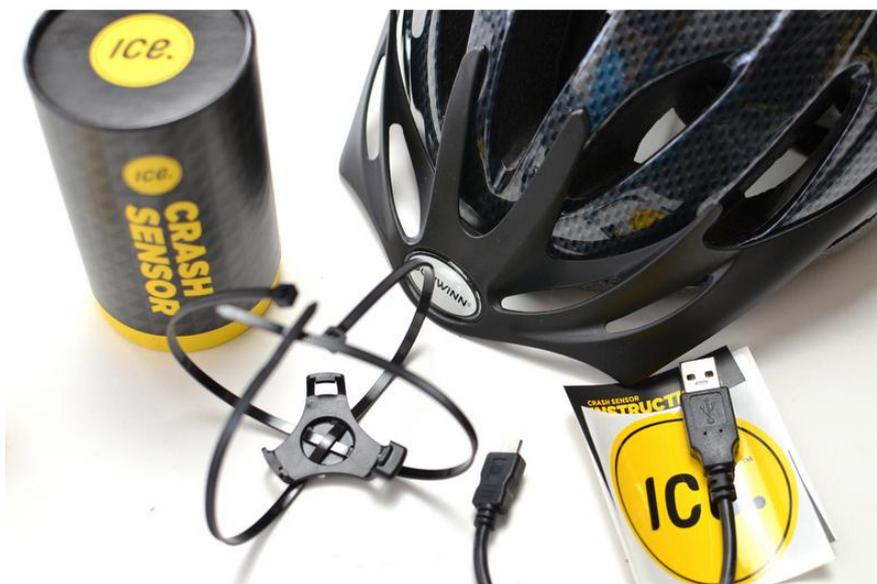
The ICEdot attaches to your helmet with a bracket and zip ties, and the device charges via micro USB. The pack also contains stickers with your ICEdot ID for placing on your license in your wallet etc.
