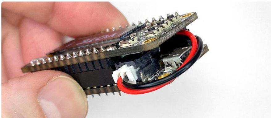
Reconnect the OLED Featherwing to the Feather while being careful not to pinch any part of the battery in the process. Lipoly batteries are somewhat delicate and can be dangerous if punctured!
