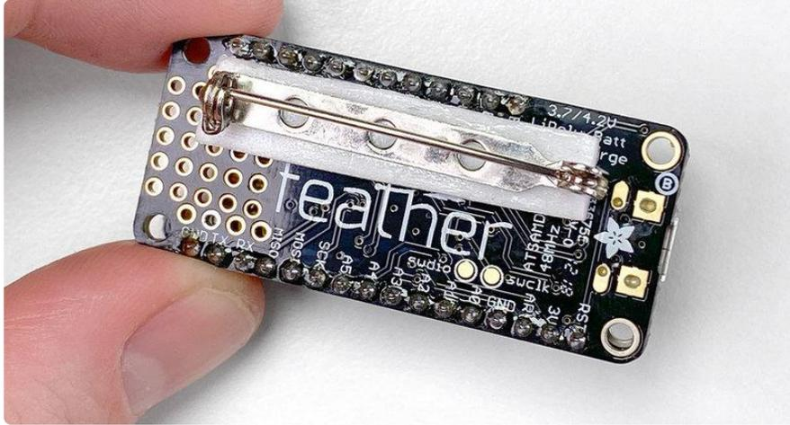
Peel the protective layer off of the pin back's adhesive side and attach it to the back of the Feather. Placing the pin back as seen above will help prevent the pin from being top heavy and tipping forward while in use. Press the pin back firmly in place to ensure it's secure.
