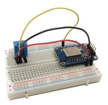
As mentionned before, you will see that I used a DHT11 sensor on this picture. However, the code you will find on GitHub is made for the DHT22 sensor, and I really suggest using a DHT22 sensor as it is more precise.
