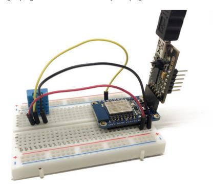
Open the code with your Arduino IDE, and select 'Adafruit HUZZAH ESP8266' from the Tools>Boards menu of the Arduino IDE. Also select the Serial port corresponding to the FTDI board you are using.
