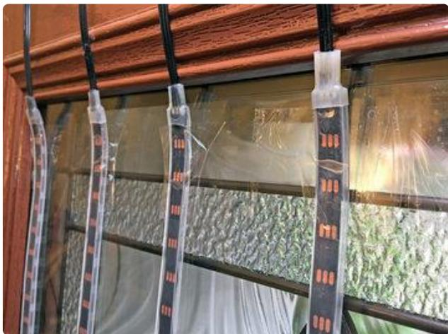
The strips are held to the glass using clear packing tape...both top and bottom, because the strips tend to curl a little otherwise. Originally I thought the JST wires would be bearing the load, but no, tape handles it fine.
