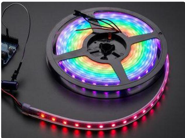
With an architectural-scale project like this, we can use regular-width, 60-pixels-per-meter NeoPixel flex strip. Fortunately this is the most common variety around!
