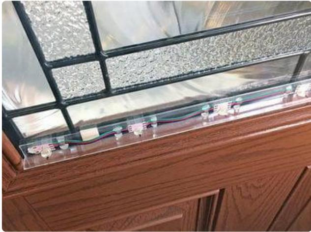
My “splat” pixels were strip-end cuttings from prior NeoPixel projects. Originally I was going to glue these to a strip of molding or maybe a dowel, but the local hardware store had this clear “L” corner protector stuff. I cut it to length for the window, hot-glued the pixels in place, and held it to the window with a couple small pieces of double-stick foam tape.
