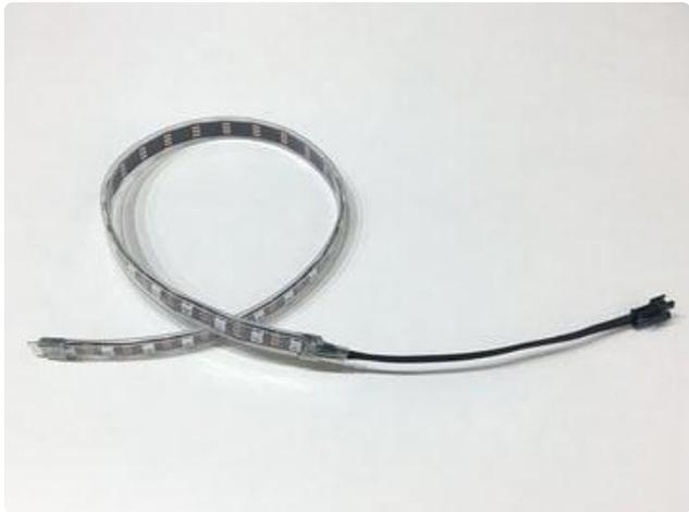
Even though my icicle lights will be inside the window, I wanted to keep the weatherproof covering in case these are re-used in different situations later. This requires sealing the ends of the strips with hot glue and 1/2" clear heat-shrink.
