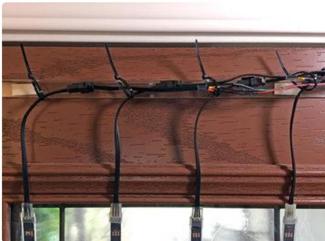
Up top, the same plastic “L” channel (with holes drilled at suitable intervals) supports the wires, held with zip-ties. The Feather hardware is out of frame to the right.
