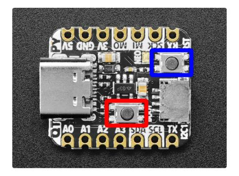
To enter the bootloader, hold down the **BOOT/BOOTSEL button** (highlighted in red above), and while continuing to hold it (don't let go!), press and release the **reset button** (highlighted in blue above). **Continue to hold the BOOT/BOOTSEL button until the RPI-RP2 drive appears!**
