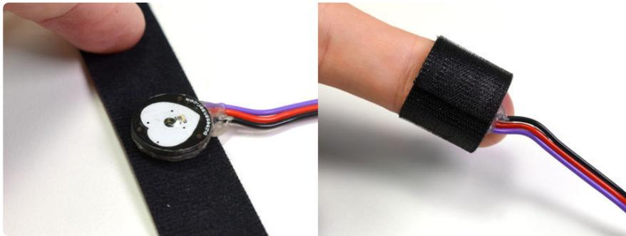
Once the sensor is secured, connect the Circuit Playground board to power via the USB or battery connector and you should see the two LEDs near the USB jack begin to flash in time with your pulse.
