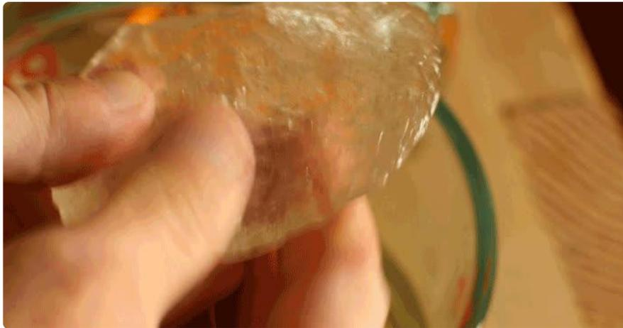
Next, fold the flat piece of plastic over the chisel as shown in the video below. Make sure to leave enough padding on the edge of the chisel so it won't cut through the end of the guard. You may want to dunk the flat piece back in the hot water for a minute before doing this step to make sure it is easy to fold over the chisel.
