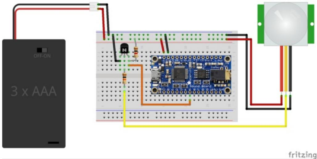
Most of the wiring is relatively straightforward, just connect component grounds to battery ground and component VIN/voltage input to battery positive voltage.
