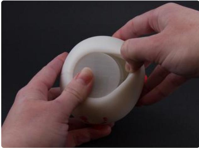
Stretch the outside casing off of the internal plastic housing.
