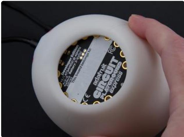
Press the CPX into the groove, starting with the section near the USB. Apply a constant gentle pressure to keep the CPX in the groove as you go. Gently stretch the lamp housing around the CPX until it's entirely fitted into the bottom of the lamp.
