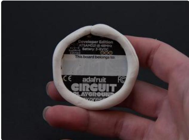
Open up the packet, take the Sugru out and make it into a snake the right length to circle around the Circuit Playground Express. Place it around the back of the CPX, and then press it down onto the base of the lamp.
