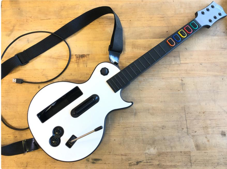
Thanks to the Wii Accessory plug on the controller, we can make all of our connections without disassembling the guitar. The plug hooks up with the Wii Nunchuck breakout adapter very simply!
