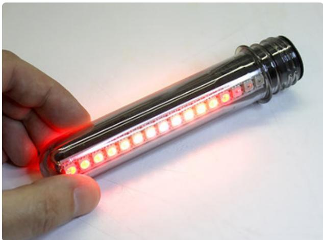
Fire it up, confirm everything still works. Screw on the cap and make sure it doesn't accidentally trigger the mode button or power switch.
