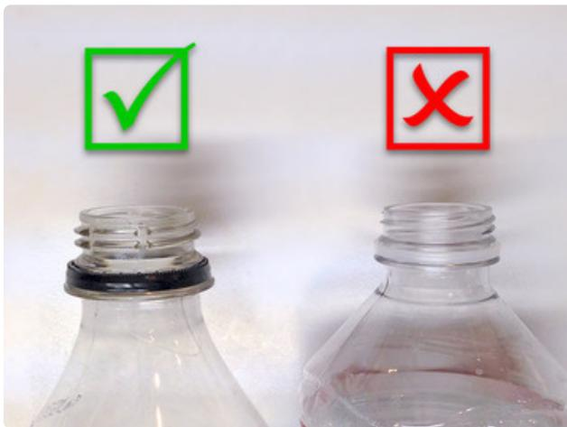
Trouble finding preforms that fit the 3D parts? Not to worry! Some small soda or water bottles occasionally work. Look for one with the traditional coarse soda thread...many varieties of bottled water use a finer thread that won’t work for this project.
