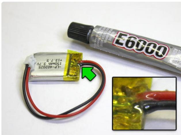
Before doing any soldering or other work, do this: using a small dab of E6000 glue or 5 minute epoxy, reinforce the wires coming off the LiPoly battery. We'll make a sharp bend there later and don't want the wires breaking off.
