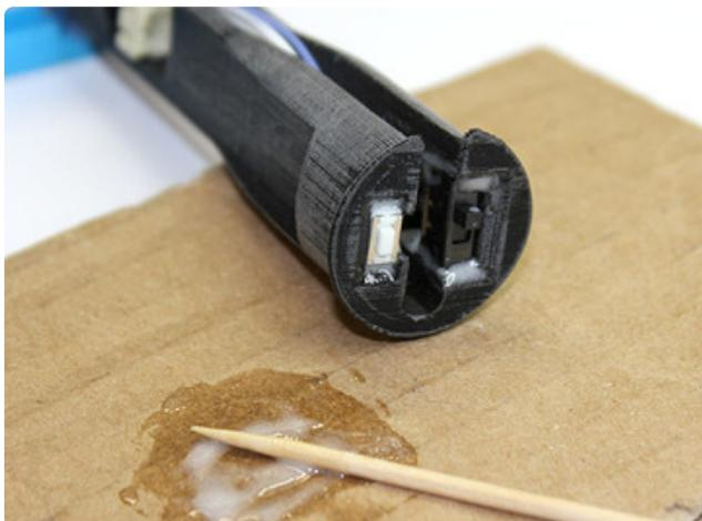
Glue the power switch and mode button in place. This step really calls for epoxy, not E6000.
