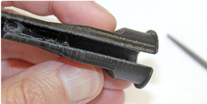
A lithium-polymer battery will slide in there later. Puncturing LiPoly batteries is one way they can catch fire, hence the extra attention to removing plastic nubs here.
