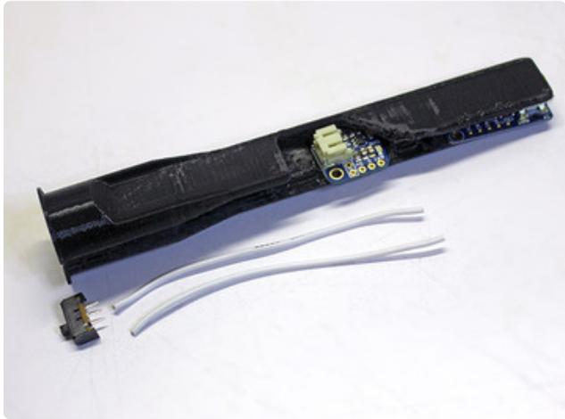
Cut two **3-inch (75 mm)** — or slightly longer — pieces of **26 gauge silicone-insulated stranded wire** and strip about 1/8" insulation from one end (to match the pins on the switch). Give the bare ends a twist and “tin” the wires with a tiny bit of molten solder.
