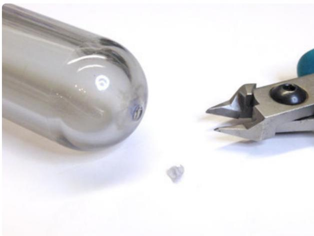
Clip or sand off any plastic “sprue” protruding from the end of the preforms. These are sharp and will hurt if caught in motion!
