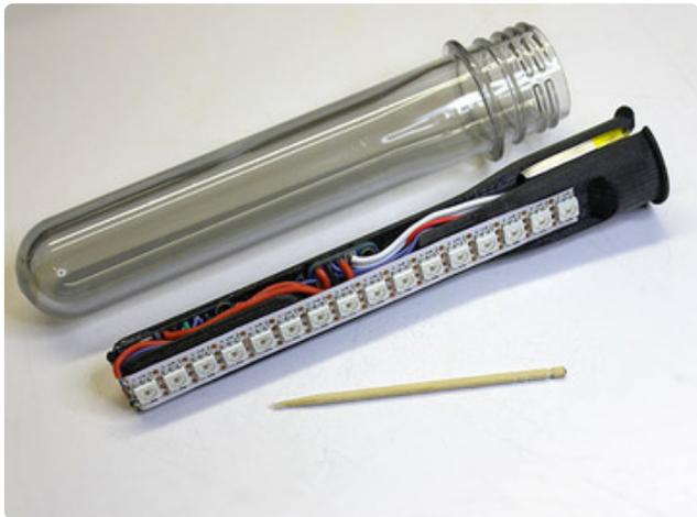
Once the glue is completely dry, using a toothpick or other nonconductive tool to carefully pack all the wires inside.
