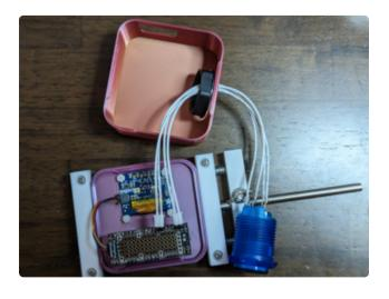
Take two of the quick-connect wire harnesses. Press the ends gently but firmly onto the arcade button. Then pass the wire harnesses through the hole in the case, through the threaded nut, and attach them to the right angle headers.
