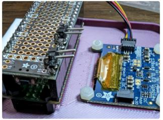
Solder two 2-pin sections of 90 degree header:
