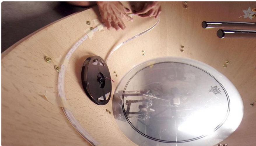
You can choose how deep you want your lights to be in the shells. For the drum kick, we positioned them away from the drum pedal so it's brighter when facing an audience. In the tom toms and the snare, the LEDs are positioned closer to the drummer, but you can mount them closer to the bottom for the audience. You can use paper tape to keep the strips mounted to the inner lining. We can do this after we solder wires to the NeoPixel strips.
