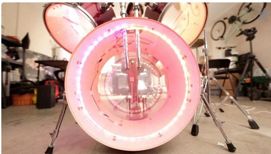
Once you have all of the parts mounted and secured to the shells, play and test out each piece. If you have issues with the LEDs, make sure your battery is fully charged and check your alligator clip connections to see if any wires are touching. The amount of sensitivity will vary depending on where you position the mic sensor.
