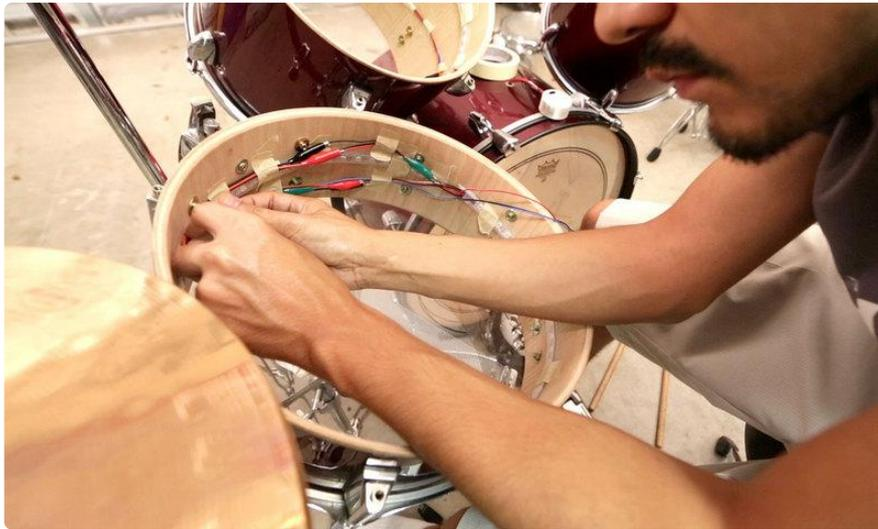
The NeoPixel strips will be mounted to the inner lining of the drum shells. You can measure and cut the length of an LED strip needed to cover the whole shell. Use the indicator on the strip to cut them properly. Position the first LED pixel closest to the air hole of the shell. The wires at the end of the strip should remain inside the shell.
