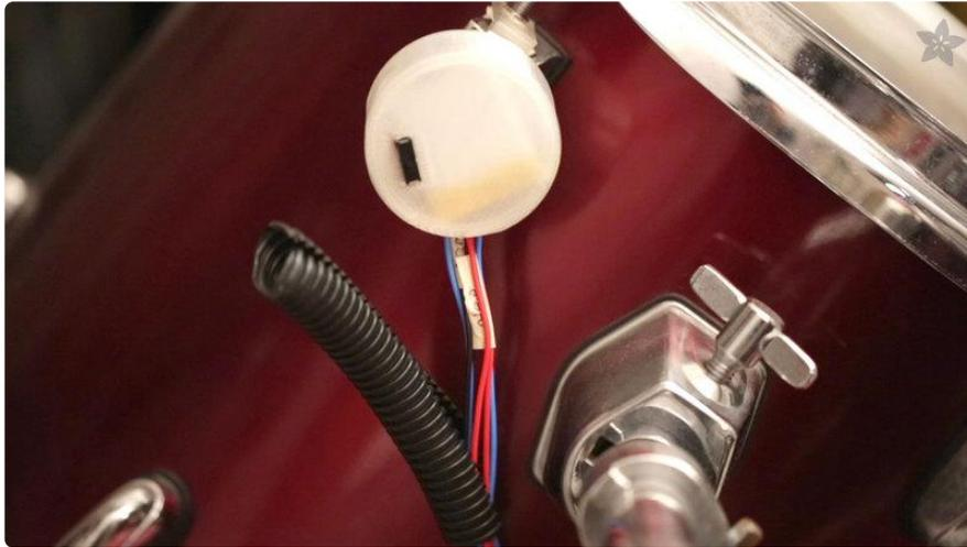
We used pieces of cable tube organizers to protect the exposed wired. You can also use shrink tubing for a more permanent finish.
