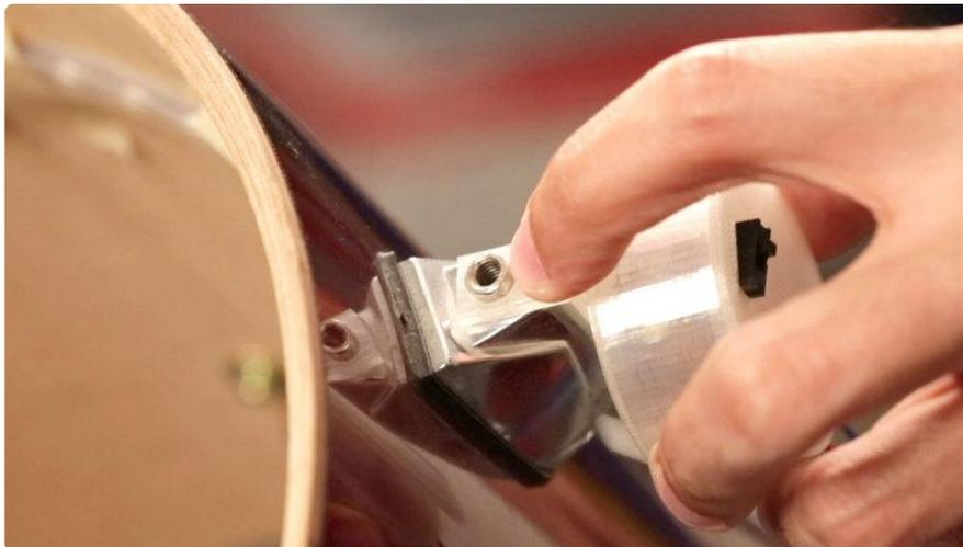
Attach the hanger to the back of the case with a piece of double-sided foam tape. Position the hole on the hanger above the shell pin and press it down to mount it into place.
