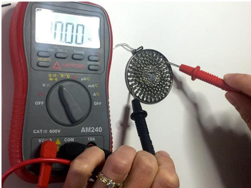
For the capacitive touch pad to work when it's connected to your pendant, you'll need to be sure to use a pendant that conducts electricity. Use your multimeter to test and be sure your pendant is conductive.
