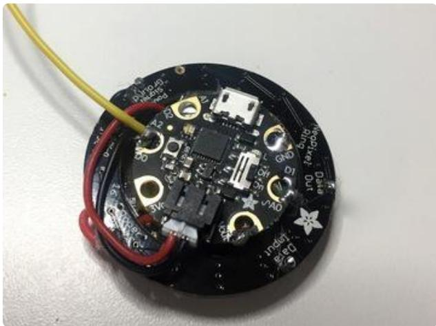
Solder a 2" wire to gemma's pin D0. This wire will connect Gemma's capacitive touch pad to your metal pendant front to activate the capacitive touch features.
