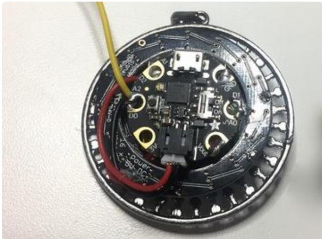
Place the Gemma on the back of the pile, with the switch facing up. Be sure the battery wire can be pulled out easily and replaced -- you'll need to unplug this for charging. Once it's all aligned, glue all the components together with E6000 glue or epoxy.
