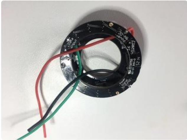
Pull the three loose wires through so they come out the back of the larger ring. Trim the wires and solder them to the Gemma: red to Vout, black to GND, and your data wire to D1.
