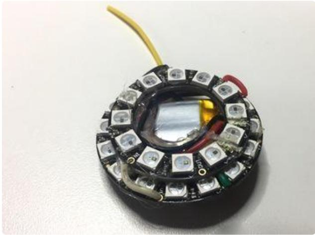
Set the battery inside the large ring and nestle it against the back of the smaller ring. Center the rings so the LEDs show as much as possible.
