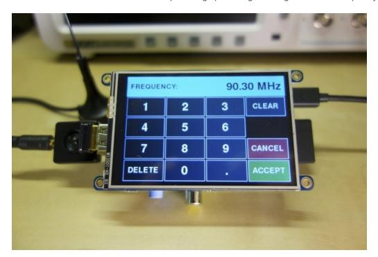
You can change the center frequency just like inputting numbers in a calculator. Press the **CLEAR** button to completely erase the current frequency value, enter new digits by pressing numbers (or the decimal point), and delete the last digit by pressing **DELETE**.
