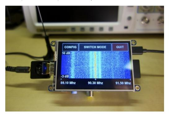
The waterfall plot displays intensity over time. Each row of the plot represents a point in time, and each pixel color in a row represents the intensity of the signal at that frequency. Pure blue pixels are the minimum intensity, pure red pixels are the maximum intensities, and a gradient of blue-cyan-yellow-red represents in between intensities.
