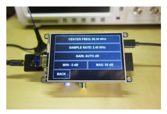
Press the **CENTER FREQ** button at the top to bring up a dialog to change the center frequency:
