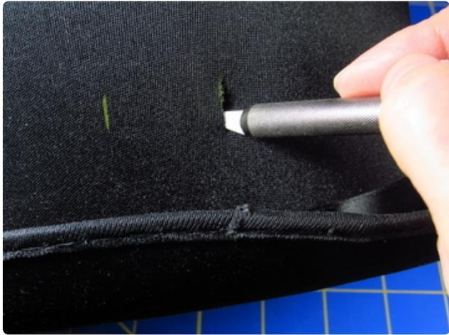
If you want to hide the excess wires inside the hat, mark two small holes on either side of where you want to place the Gemma LED. Leave enough room so the wires don't have to bend straight down, to avoid straining and possibly breaking them.
