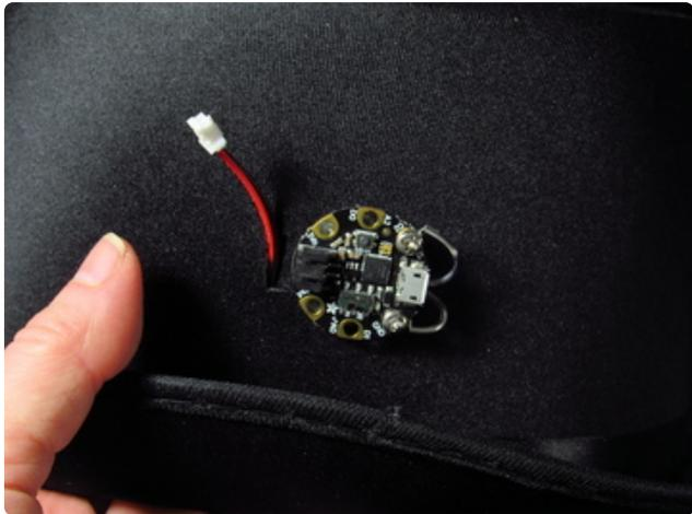
For the battery pack wire, cut a small flap to fit the JST plug through. Press the flap closed around the wires when you're done.
