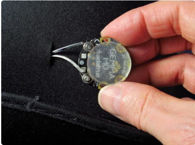
Then carefully cut a slit for the light wire. (A [ceramic craft knife \(http://adafru.it/4306\)](http://adafru.it/4306) is safe enough for kids to do this themselves, with adult help.) Thread the end of the light wire through the slit.
