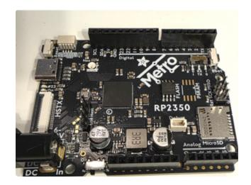
Turn the board over and remove the material securing the pins. Now there is a new 4-pin header.
