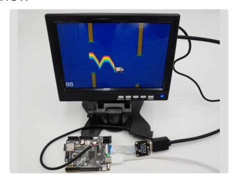
The Metro RP2350 makes a perfect little game console. The on-board HSTX combined with a DVI breakout can output to a standard television or computer monitor for the display. The broken out USB host connections make it easy to take input from a keyboard to control the game.
