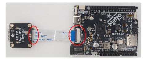
Get the HSTX cable. Any length Adafruit sells is fine. CAREFULLY lift the dark grey bar up on the Metro, insert the cable silver side down, blue side up, then put the bar CAREFULLY down, ensuring it locks. If it feels like it doesn't want to go, do not force it.
