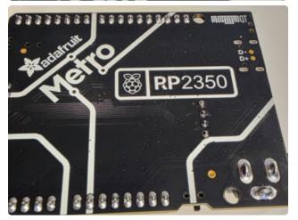
Put the short end of the header into the holes in the Metro marked USB Host and secure them with putty, blutack, tape, etc. Turn the Metro over and you should see the header barely poking out of the bottom of the board. If the pins stick through a great deal you may have the header pins upside down, double check the short end is sticking into the board.
