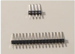
The USB Host pin connections are highlighted on the Metro image to the left. You will need a small piece of standard 0.1 inch male header, with 4 pins, to fit the holes.
