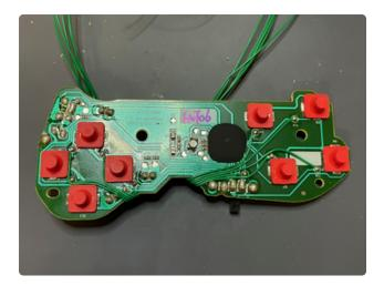
Strip the insulation from the tip of each wire and solder them to the test points.
