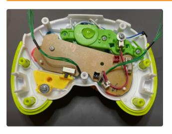
Tuck the speaker wire over to the side to make room for placing the KB2040.
