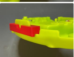
Start by placing the top cutting jig onto the top section of the back half of the shell.
