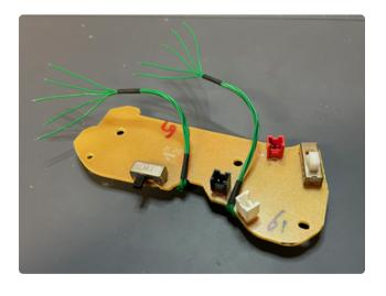
Place a small bit of heat shrink around the two groups of wires. This will help keep things nice and tidy.
