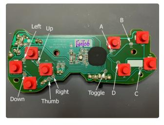
Pre-tin all 10 test points with a bit of solder.
