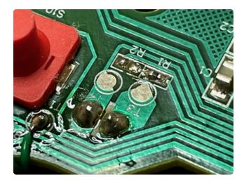
By removing the R2 resistor, the rear toggle switch can be used to turn off/on the speaker.
