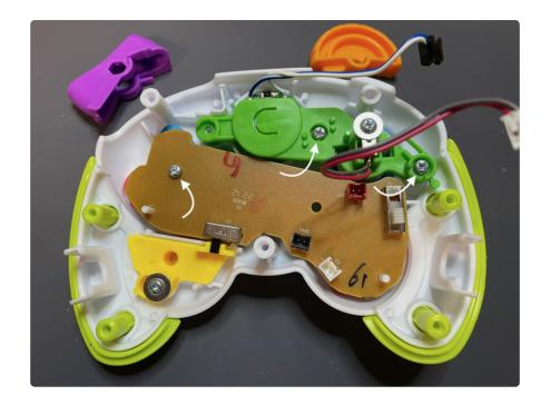
Pay close attention to the positions of the internal screws, as there are more screw holes than actual screws.
