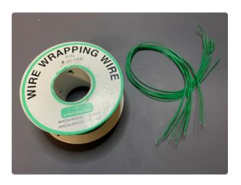
Using 30AWG wire wrapping wire, cut 10 wires at roughly 10 inches / 25.4cm to allow for plenty of slack to work with.
