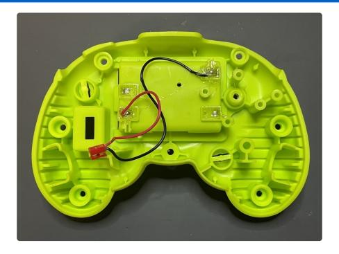
Lastly, there are three more small Phillips screws that need to be removed inside the controller. Two of these screws secure the speaker bracket, while the third one holds the PCB in place.
