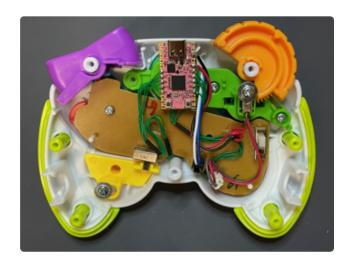
Once soldered, reconnect the speaker wire and gently tuck the newly added wires into the center cavity between the boards.
