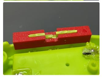
If cutting without the 3D printed jig, then start by trimming off 5mm of the tab in the photo below. Then hold off on cutting the 9x3.5mm USB-C slot until the final assembly.
