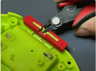
Using angle cutter pliers, carefully trim off the plastic above the jig.
