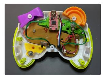
Then press the KB2040 into place with the USB port sitting on the white edge and the board within it.
