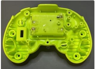
Since the existing batteries are no longer needed, begin by carefully trimming the power wires as close to the back shell as possible.
