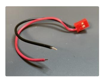
Next, ensure the black and red wires are of equal lengths, and carefully remove a small portion of insulation from their ends.
