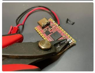
To remove, start by using angle cutters to gradually cut the connectors two front legs.
