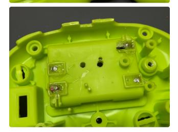
So two roughly 3.5mm holes need to be drilled into the battery compartment for these two buttons.
