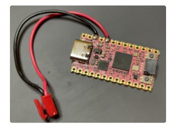
Now, proceed to solder the red wire to the 3.3V pin (marked '3V') and the black wire to the ground pin (marked 'G') on the KB2040.
