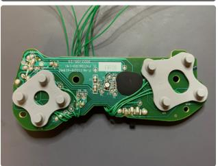
The same steps apply except the button silicon pads will need to be temporarily removed to access the solder points if you have the variant with large connected elastomer pads as shown here.
