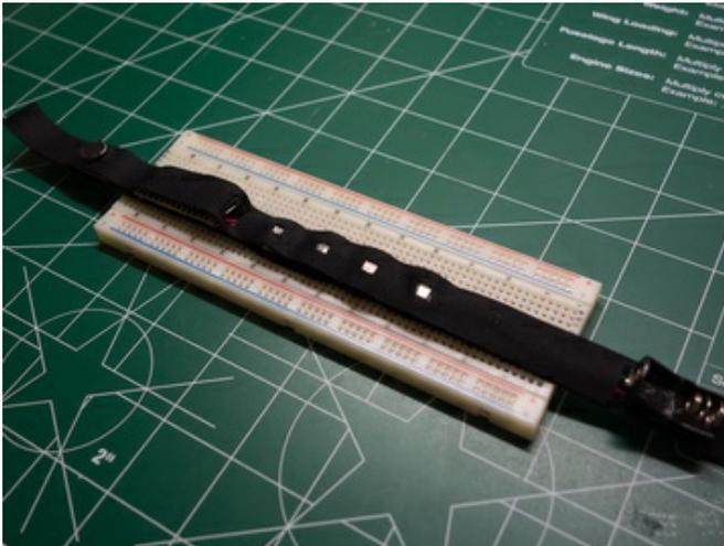
You can also see in the second image the hardware can be put together into a simple wearable collar. I took two pieces of velcro and sandwiched the hardware in the center. Holes were cut out to show the LEDs, USB mini port, and microphone.
