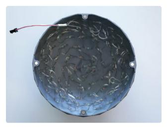
Install LED strip to Top Half Start attaching the second LED strip to the top half of the sphere beginning with the first LED hot glued to the edges. Then, continue attaching in a spiral direction.
