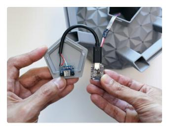
Connect USB to QT Py Grab the USB-C cable from USB-C breakout that's secured to the bottom cover and plug it into the QT Py's USB-C port.
