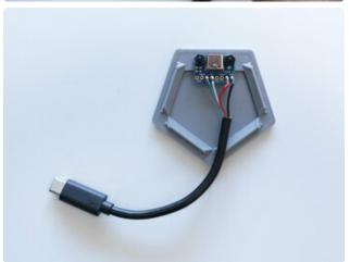
Insert and fasten the screws through the mounting holes. Use the hex nuts to secure the USB-C breakout.
