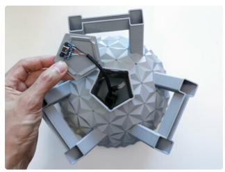
Install QT Py & BFF Insert the QT Py and NeoPixel BFF into the center of the bottom half.
