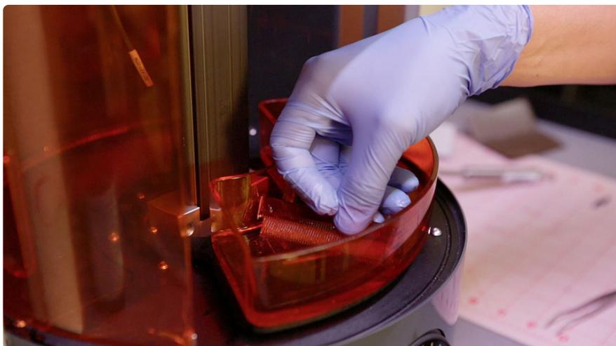
Keeping the resin tank clean is important. As prints fail, material builds up and floats around the tray. These can be difficult to spot, so we can use a hair comb to filter out any pieces left behind. Use tweezers to fetch out any bigger pieces.
