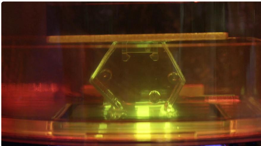
The ember printer uses a cure and peel technique. This exposes and separates for each layer to create a high definition part.
