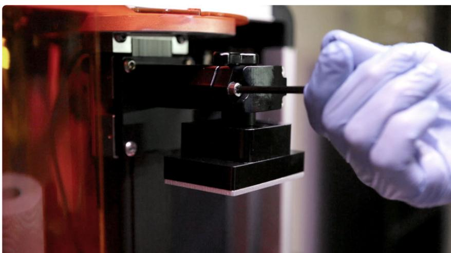
We'll need to relevel the build head before starting a new job - mainly because it misaligns after removal. So we can loosen a the build plate and move it up, and then we'll tighten up the screw.
