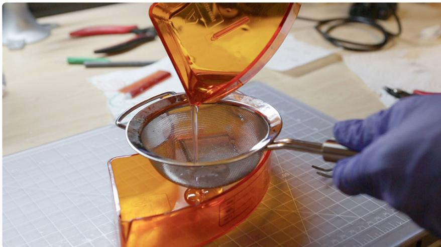
If there's a lot of bits and pieces, use a fine mesh strainer to quickly filter out smaller debris into the second tray. The build head is easy to clean after each print, just wipe off any remains.
