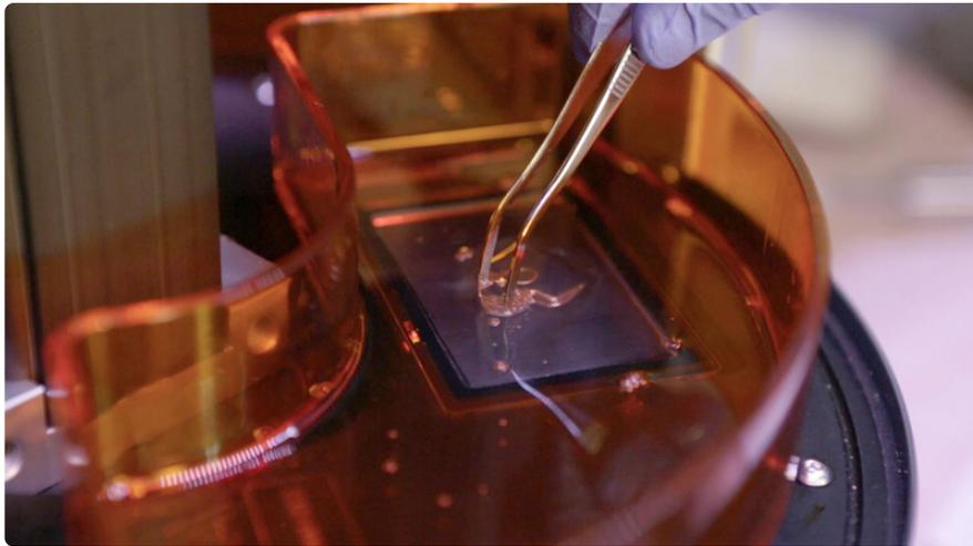
Carefully swipe around the edges of the resin tray window and remove any build up.
