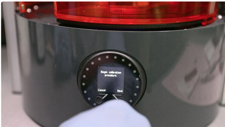
Then we'll initiate the leveling procedure - It'll start homing the build head down until it reaches the resin tank window.
