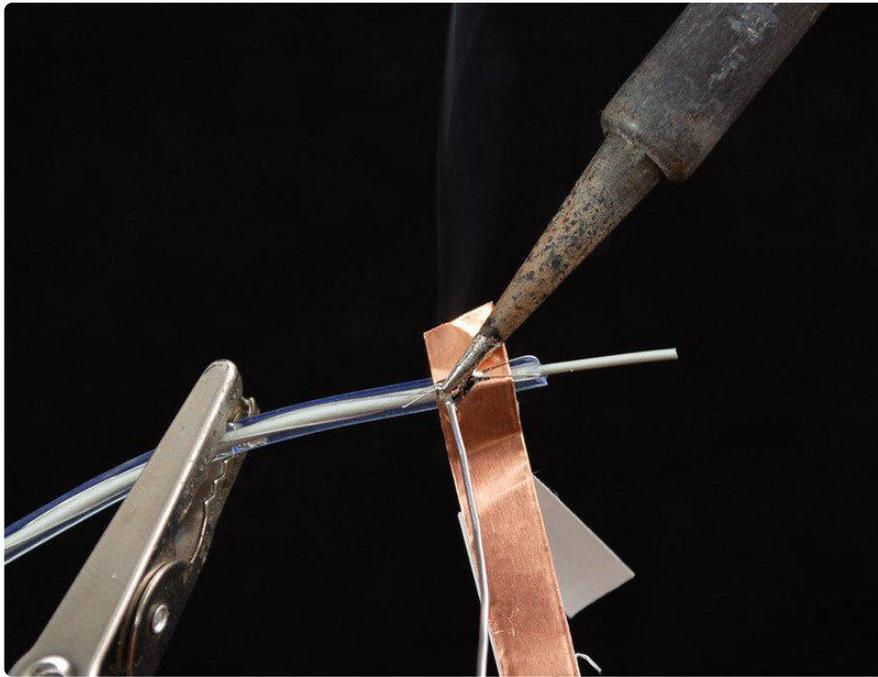
Solder demo - show the EL soldering process start-to-finish and explain how to decide when to solder a new branch and when to just mask a section of EL with heat shrink.
