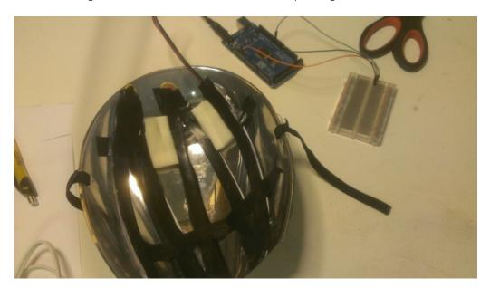
Now on to the Trinket end of things... if you wrap up all the wires from your trinket to the mask with electrical tape, then the trinket can sit above your head while wearing the mask. The switch can go along the side of the mask, down near your ear, and sit on the inside of the mask. The battery is easily taped right along your forehead, where it will stay put.
