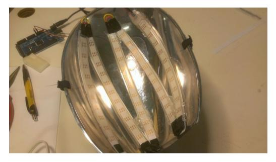
To make it easier to see out of the mask, you can also line the back of the strips with electrical tape...
