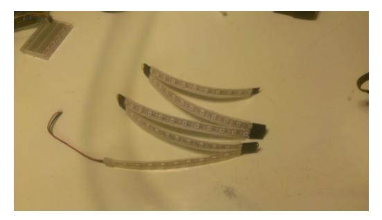
This is the longest and hardest part of any NeoPixel strip project... use an exacto knife to cut the strips exactly in the middle of two adjacent neopixels (you'll see a dotted line on the PCB), and then solder wires to the pads from each strip to the next one. Make sure all the data arrows are pointing in the same direction, for a constant flow throughout the strip.
