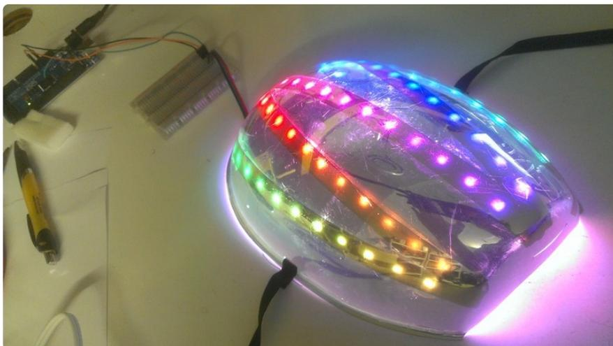
Next, it's time to glue this into the mask. But first, turn on the Pro Trinket again, and make sure everything is working! If it isn't, you'll have to go back and fix some broken solder joints.
