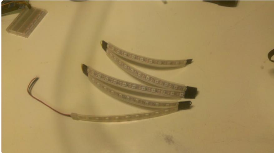
This is the longest and hardest part of any NeoPixel strip project... use an exacto knife to cut the strips exactly in the middle of two adjacent neopixels (you'll see a dotted line on the PCB), and then solder wires to the pads from each strip to the next one. Make sure all the data arrows are pointing in the same direction, for a constant flow throughout the strip.
