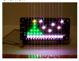
The Feather platform has really gotten my attention recently, especially since its move to using the ATSAMD21 MCU. This is a powerhouse chip based on the ARM Cortex-M0+ core. The other great thing about Feathers is the large (and constantly growing) ecosystem of add-on boards, called FeatherWings (https://adafru.it/Ci1).
