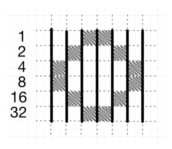
Using the numbers beside each row (which are the values corresponding to each bit), add up each column using 0 if the pixel is off and the corresponding row/bit number if it is on. Like so:
