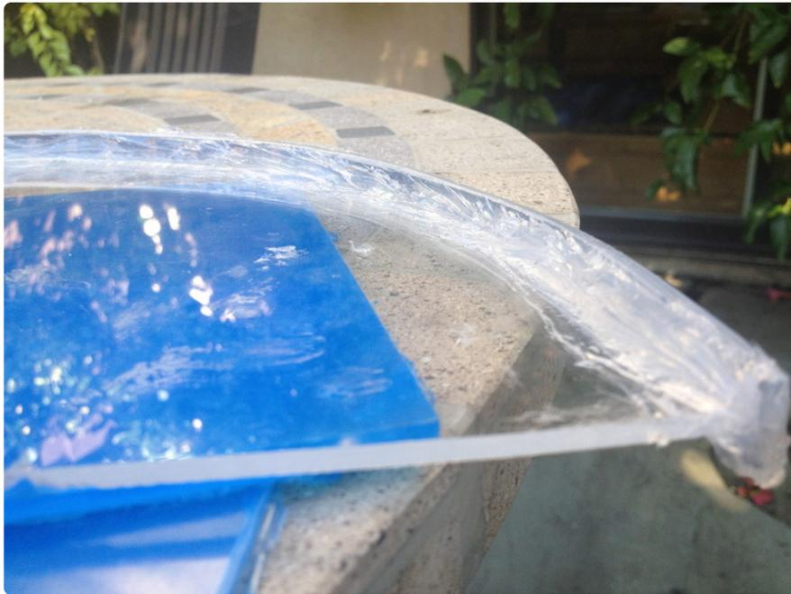
Set the acrylic fan on top of some supports so its edge is hovering about 1/4" from the table. (The leftover acrylic you just cut off works great as a support). Line the Dotstar strip against the edge so it's centered both up and down, and left to right.
