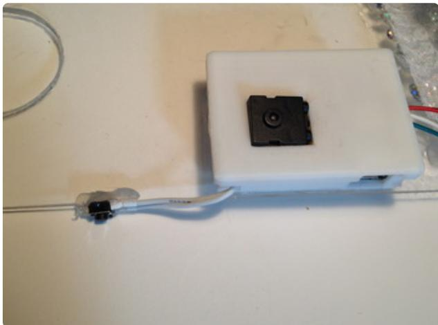
Plug the battery in and pop the lid onto the enclosure with the on/off switch positioned inside the hole.
