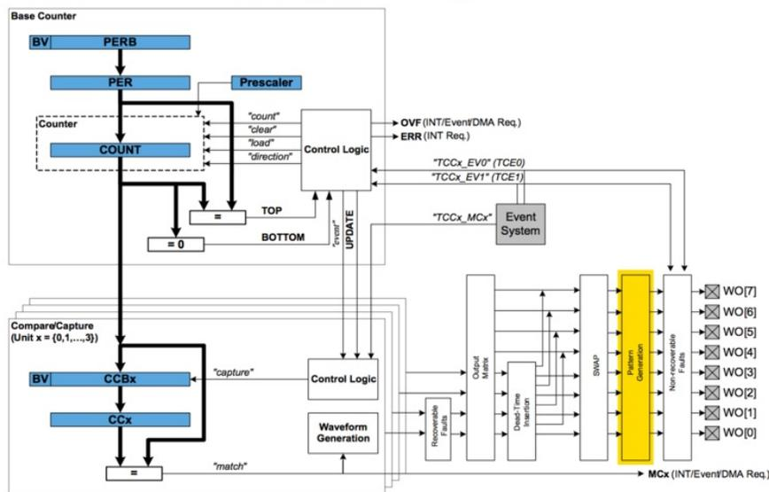
After a lot of trial-and-error, we found that this was indeed a workaround for the DMA-less GPIO output! It only provides 8 concurrent output bits (vs. up to 32 bits for the GPIO ports), but for many applications that’s sufficient.
