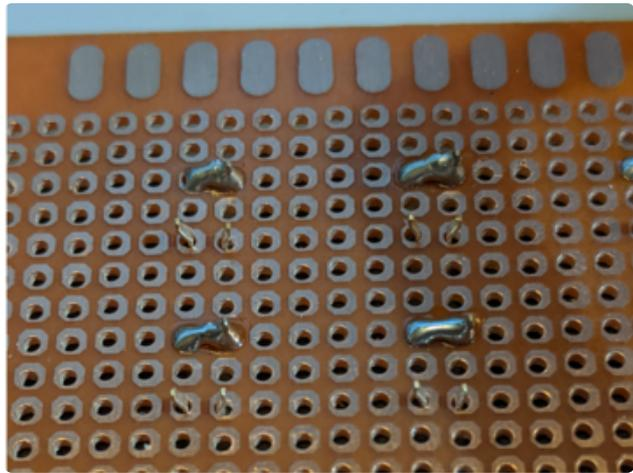
Flip the board over, the next task is to complete the "row wiring". There is already an internal connection between pins 1 and 2, and pins 3 and 4 that will be taken advantage of. (then, when the switch closes, all of 1, 2, 3, and 4 are momentarily connected)
