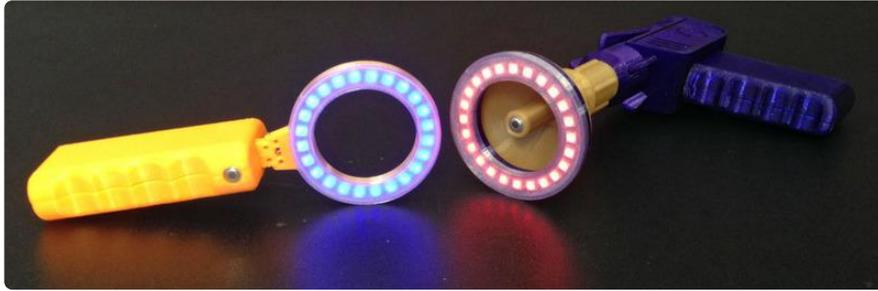
In this project we'll use a temperature sensor to change the color of a NeoPixel ring to create heat map photography. A cyber-tronic looking sensor measures remote infrared light making it a contact-less temperature sensor.
