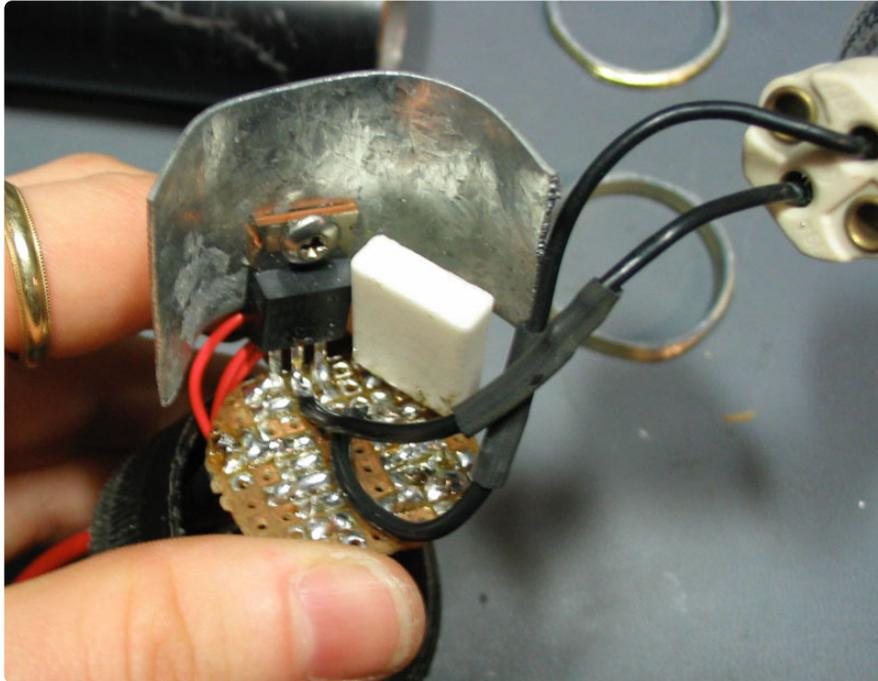
The other side of the circuit board, showing the heat sink, and the large sense resistor. Also, the lamp socket is visible in the top lefthand corner.
