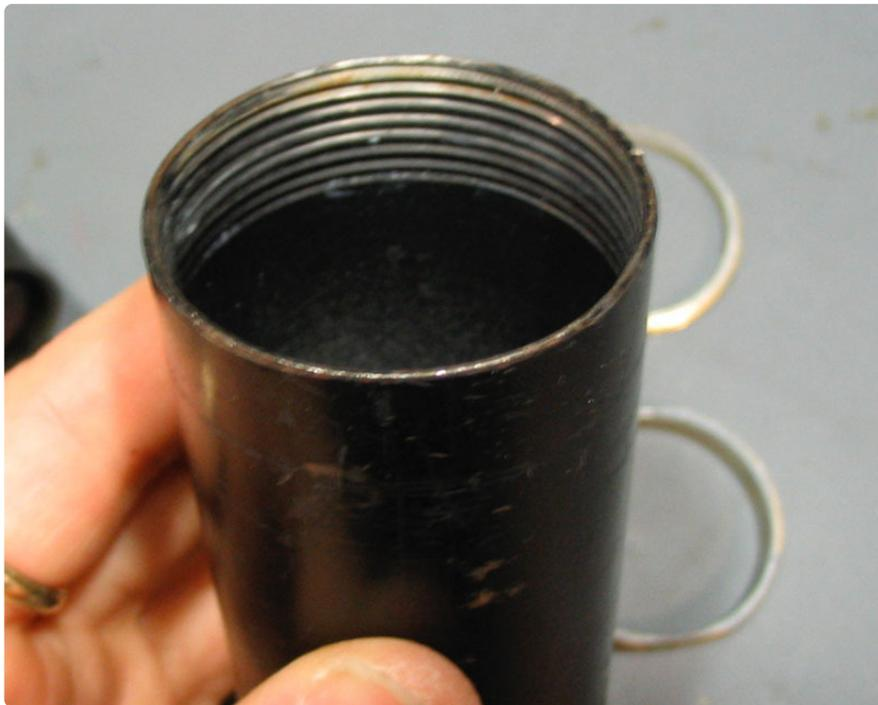
One end of the housing should have a full set of threads, the two rings are visible in the background.
