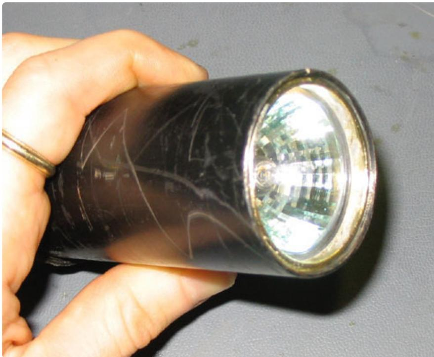
If you don't think you'll open it again, you might want to put a drop of threadlock or superglue, to keep it from unscrewing. Ducttape the cap, and hotglue/epoxy the hole where the battery wires emerge.
