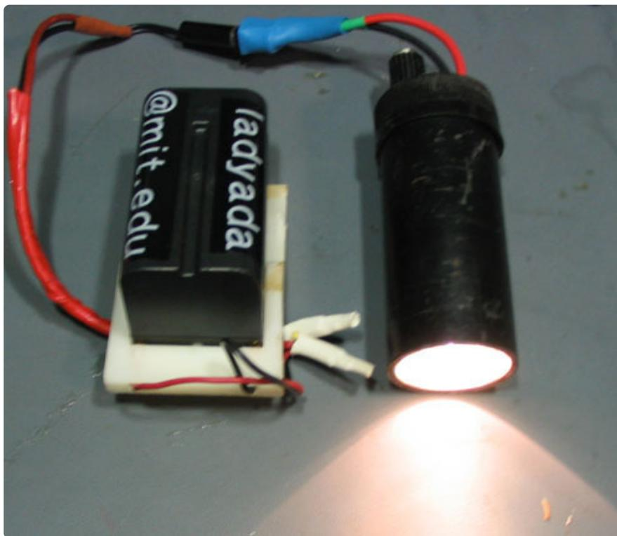
Assembled light, with 10W halogen, and 3.5Ah 7.2V lithium ion battery pack (the nice battery holder was custom made for another project).
