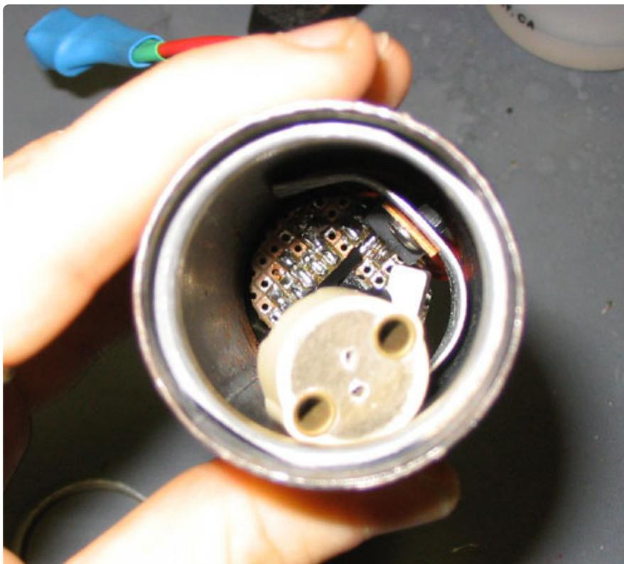
Then thread the inner ring, plug the lamp into the socket (or solder it in).
