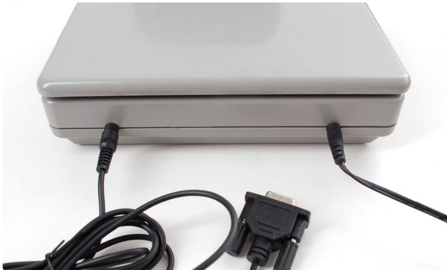
If you are trying to connect to a microcontroller/microcomputer, you can use a male DB-9 and then use a MAX232 or similar to convert from the +-10V inverted serial that comes out of the cable and convert it to plain 3.3-5V TTL serial
