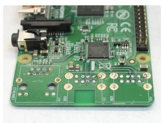
After all the pins are removed, most vias are still plugged with solder. Use the soldering iron and a vacuum desoldering tool to clear these out.
