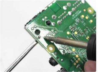
Though I have a solder reflow tool that should, in theory, be able to heat all the pins for extracting the part...in practice I was having no luck, and went back to my trusty soldering iron, heating, prying and rocking. Use whatever you have and works well for you.
