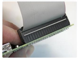
Use a spare piece of single-row pin header as a template for trimming the GPIO pins. Wedge this pin side down between the GPIO rows, then trim along the plastic edge.
