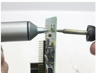
A few holes will put up a struggle...mostly the ground pins. Sometimes it's helpful to add solder (preferably the leaded type) to a hole and heat it all the way through before using the vacuum tool.
