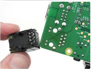
That thing about lead-free being hard to desolder? It was most troublesome with the Ethernet port LEDs, where the plastic housing would soften and deform before the solder would even melt. Fine then, let it deform, pry it up just enough to snip the legs of the LEDs. The remaining pins were desoldered with the heat-pry-rock technique.
