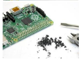
The edge of the header's plastic support can be lifted slightly using flush cutters. Be careful not to cut the pins!
