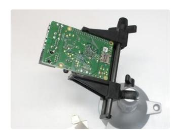
A vise is essential. This leaves both hands free...one for holding a soldering iron, the other for prying and desoldering tools.
