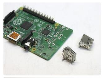
You can install one or two replacement USB ports, depending on your needs. Unlike the old stacked ports, these are single-height, so two is the maximum.
