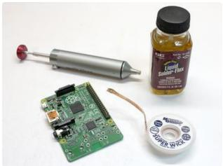
Solder wick is heated under the tip of the soldering iron and rubbed across the areas to clean...this soaks up solder like a paper towel! Do this on both sides of the board. Applying liquid soldering flux first (either the brush-on or pen applicator type) makes this process a little smoother and cleaner.
