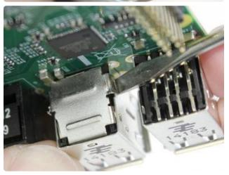
Dismantling the metal housings around the Ethernet and USB ports can help reduce the overall thermal mass when desoldering, and makes some pins easier to access. But they're destoyed in the process and can't be salvaged.
