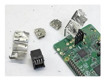
The USB ports similarly required a lot of grappling. Rather than trying to desolder the pins and pry the housing off the board, the housing was dismantled and the pins were clipped from the component side, and the schrapnel will be cleaned up later.
