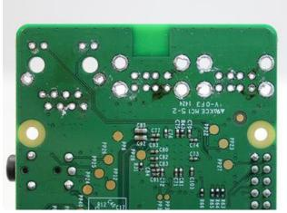
The holes are clear, but there's still a lot of solder debris on the board...this can bridge vias and cause mayhem, even if you're not using the corresponding ports.
