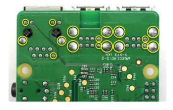
Lead-free desoldering is already tough, but a few points on the board are particularly challenging. They're connected to the ground plane, which becomes a big heat sink.
