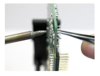
The sad remains of the ports are then cleared. As each pin is heated from the underside, it's plucked out with tweezers from the component side.
