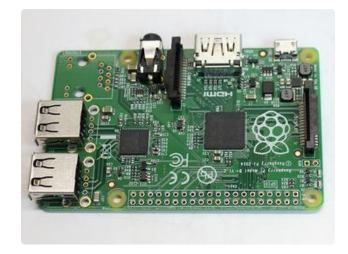
Or, if you don't anticipate using the GPIO header at all (or just need a few pins and can wire to them directly), it can be completely desoldered and removed.
