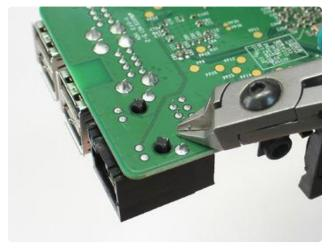
Removing parts often requires a rocking motion; heating one end while prying from the other, alternating sides. Cutting pins flush with the surface of the board reduces the amount of rocking needed...they'll clear the vias sooner.
