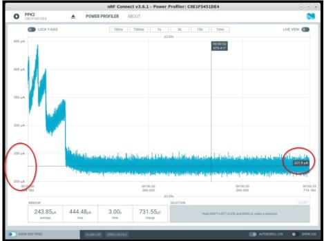
ESP32-S2 TimeAlarm Light Sleep Sample Power Consumption
