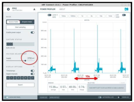
Let's zoom in on the power consumption while the program is actively running during one cycle. You can see it's using about 50mA. Note that the vertical axis scale has changed, because we're not including the big spike at the beginning of a run.
