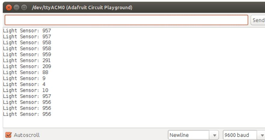
Play around with shining different lights on the light sensor and changing the distance. Also try covering the sensor with your hand, a sheet of paper, or anything else lying around (like a diary). The value can range from 0 to 1023, with higher numbers meaning more light is getting to the sensor. When you cover the light sensor, you should see the value go down.
