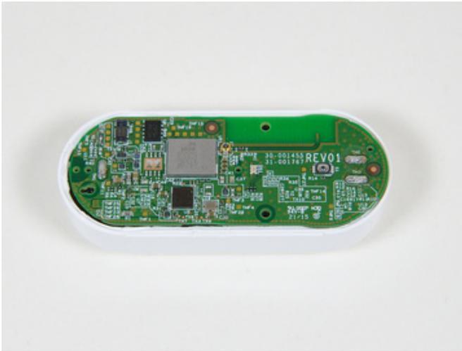
After removing the screws you will need to pry the top cover off the bottom of the Dash as it is glued firmly in place.
