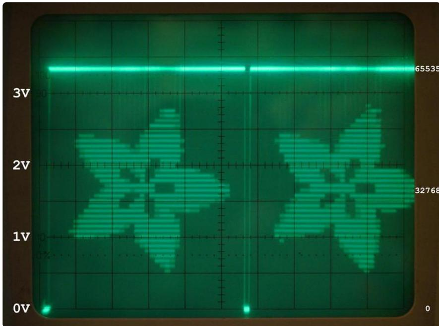
The libraries for manipulating image formats are too complex and bulky to run on the SAMD21 (M0) boards like the CPX. The data for the DAC is best prepared on a host computer as a (mono) [wav](https://adafru.it/FI0) file.
