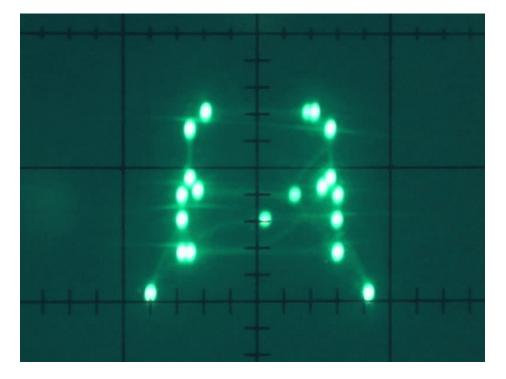
This project demonstrates two techniques for making images on an oscilloscope using CircuitPython and the analogue output(s) found on many Adafruit boards.
