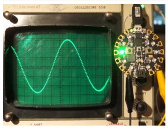
The images here show how the beam intensity (brightness) varies with sweep rate.
