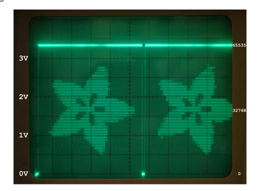
The libraries for manipulating image formats are too complex and bulky to run on the SAMD21 (M0) boards like the CPX. The data for the DAC is best prepared on a host computer as a (mono) wav (https://adafru.it/Fl0) file.
