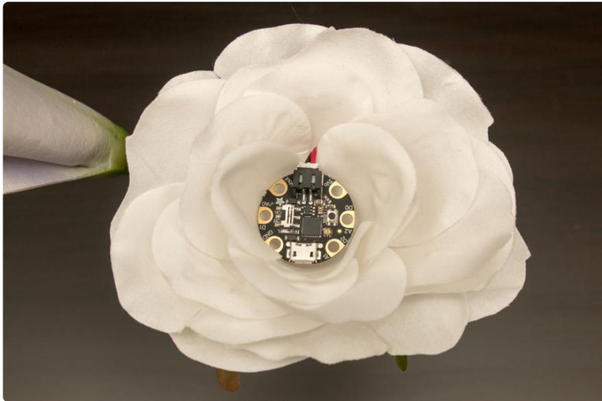
Snake the wires through the petals and down the stem of the flower. If you're using wires for capacitive touch sensing wrap them around the stem in a double helix pattern. This way when someone touches the stem they'll touch both the uninsulated ground wire and the insulated capacitive touch sensing wire:
