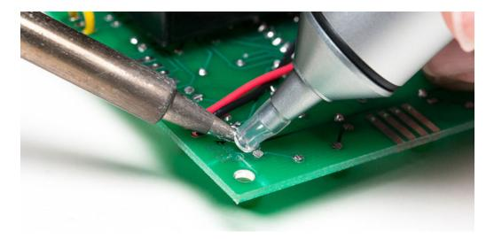
Because soldering can create such strong connections, special tools are needed to properly remove a solder joint.
