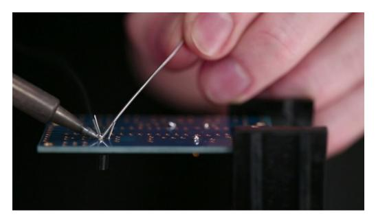
To heat both the component lead and the copper pad evenly, place the tip right here at the joint where they meet.
