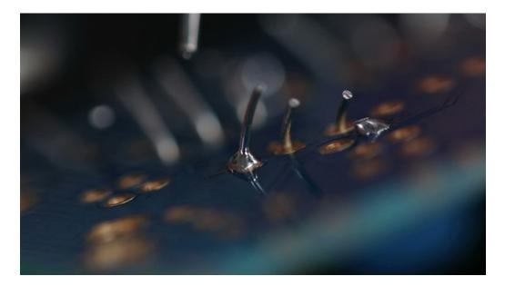
We can tell we have a good solder joint here because the surface is smooth and shiny with a slightly concave slope on each side.
