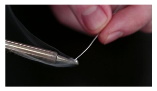
Before using a new tip, be sure to "tin" it by applying a bit of solder.
