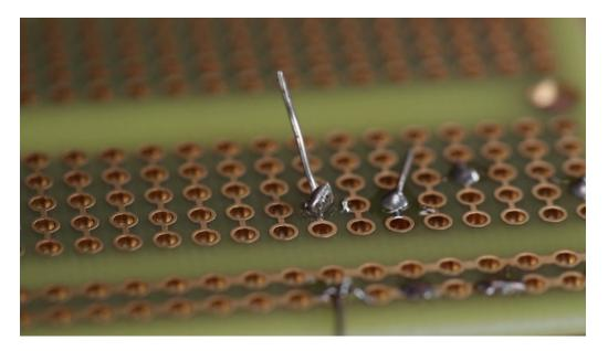
If the surface was rough or bulging excessively we may have what's called a "cold solder" joint. These occur when solder hasn't fully fused with each surface making the connection unreliable.
