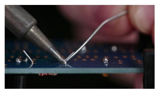
Notice I first touch the solder to the iron and then bring it down and around the component lead.
