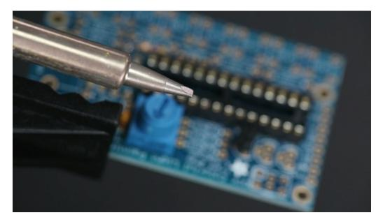
For through-hole parts like these, a flat "screwdriver" tip works well.
