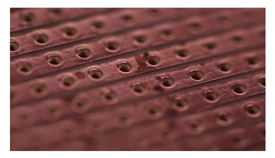
Oxidation, which can be seen here as dark spots, prevents solder from fusing with the copper surface.
