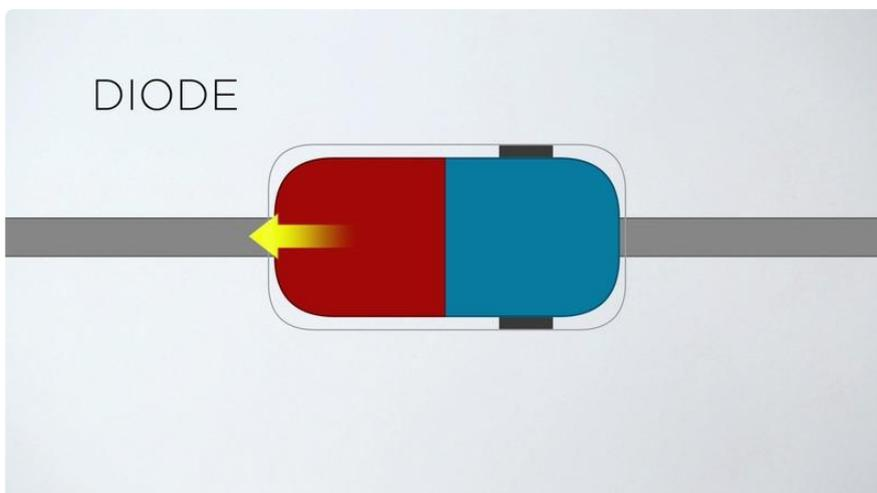
A diode uses two types of silicon stacked together to allow electrical current to flow in a single direction.
