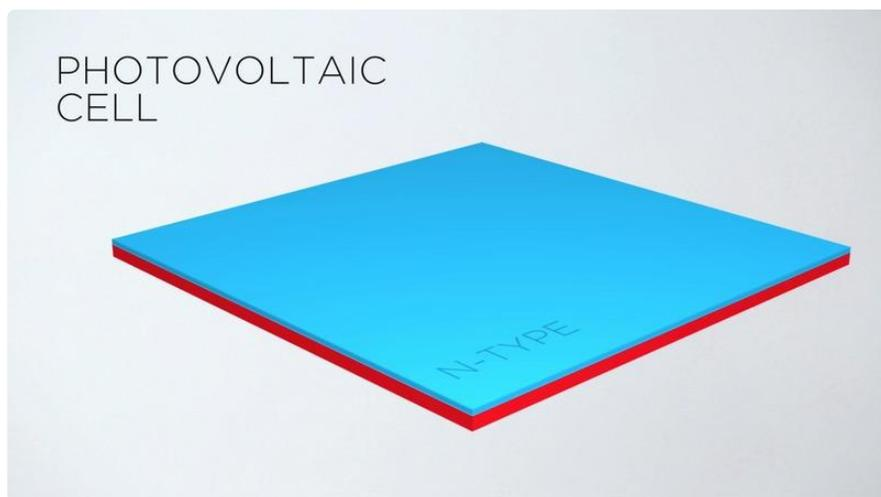
Similarly, a photovoltaic cell uses a wide, flat layer of p-type silicon covered by a thin layer of n-type silicon.
