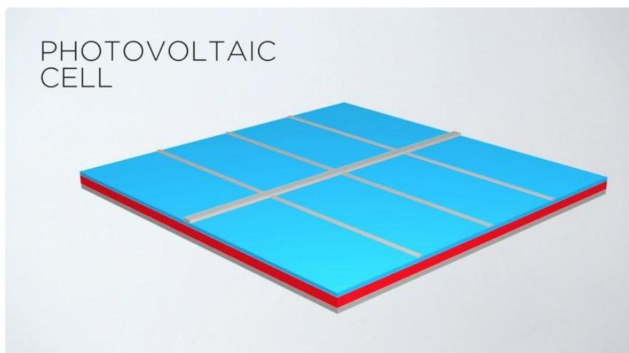
A single large flat metal conductor is connected to the bottom of the cell. And thin metal finger-like conductors are placed on top, which leaves most of the cells surface exposed to light.
