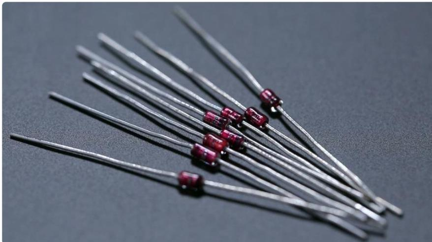
Ok - here we have a bunch of silicon diodes. They're the "small signal" type so they have glass packages - which should allow light to pass directly to the silicon.
