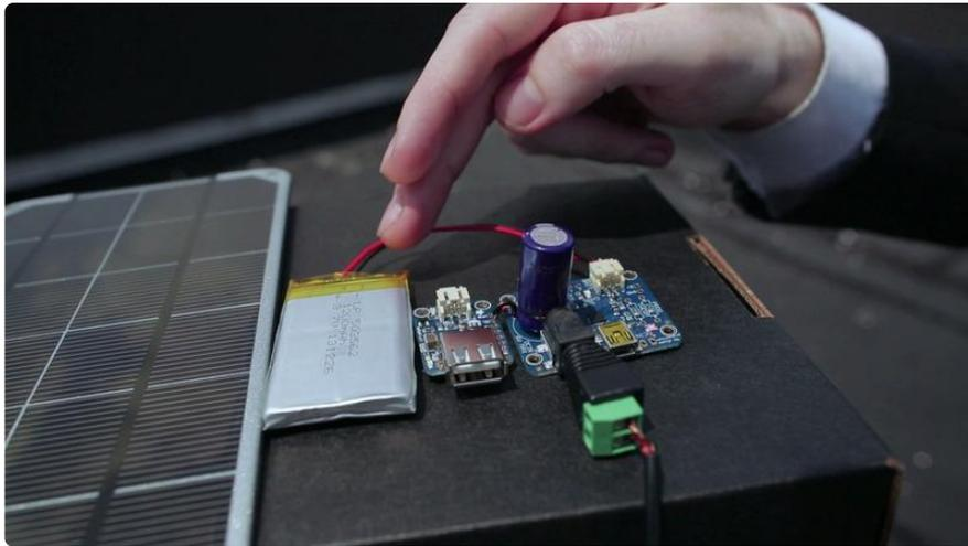
In order to charge this 3.7V LiPo battery, I'll take the output from my panel, and feed it into a specialized charging circuit ...
