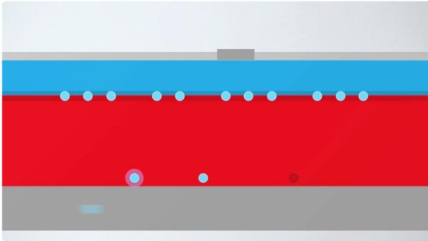
When we connect a circuit to the cell's conductors, Electrons leave the negative layer and travel through the circuit in order to reach the available holes down on the positive layer.
