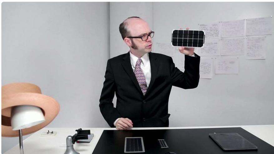
A panel like this one converts light into electricity using an array of solar or “photovoltaic” cells. These cells are surprisingly simple devices - quite similar to diodes ...
