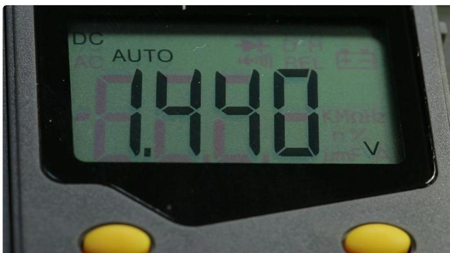
A row of 8 red LEDs produces about 1.4 volts.
