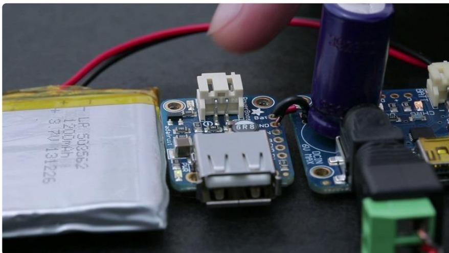
This small power boost circuit will convert the battery's 3.7 volts to a standard 5 volts suitable for use with USB devices, microcontrollers and what have you ...
