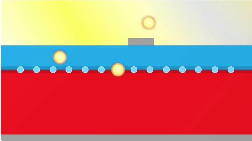
When light hits the surface of the cell, photons pass through the top layer and hit the junction between the negative and positive layers.
