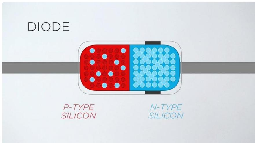
Negative, or N-type silicon, which has an excess of electrons and positive P-type silicon which has an excess of electron holes.
