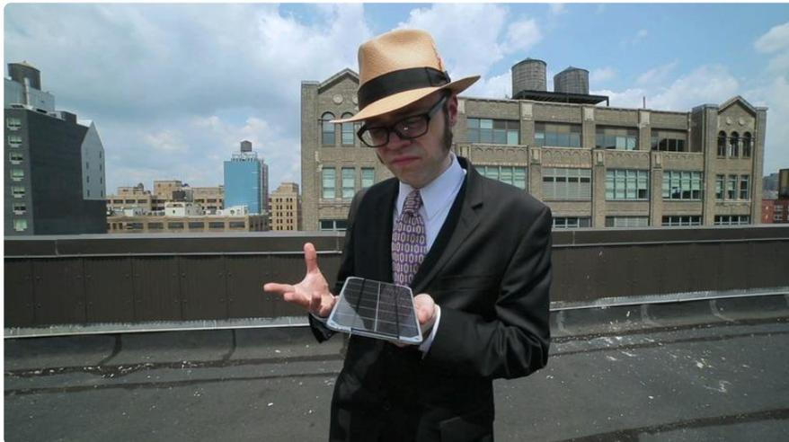
A single photovoltaic cell can provide a half a volt. My panel here has 2, 4, 6, 8, 10, 12 cells - so it can provide 6 volts.
