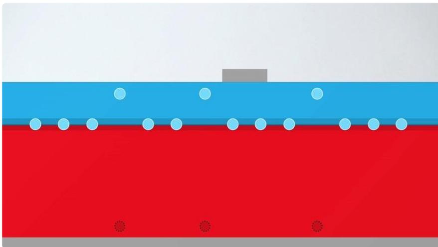
This knocks electrons out of their holes and towards the top of the cell, while those resulting holes are pushed down towards the bottom.
