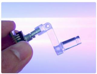
In this double-hinged crank, the clearance between the surfaces creating the hinge is 0.4mm. The diameter of the pin is 2.2mm while the minimum thickness of the part is 1.6mm.
